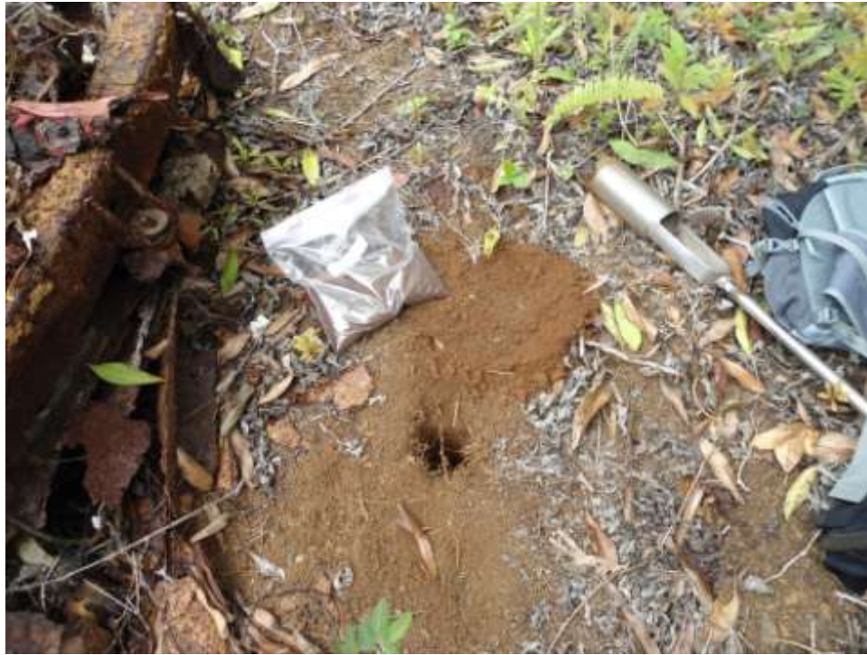
Photo 3: Sample location of second primary subsurface soil sample, which included field duplicate, and QA sample. Note Ziplock bag used for homogenization of soil. View facing down.
